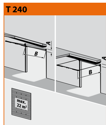
T 240 Low built-in rail system, incorporated cables + steel support profile
